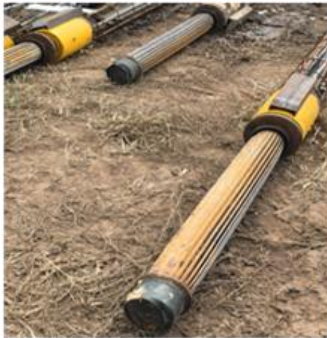
Fig. 3 Photo of the EBs and BD before pile construction.
