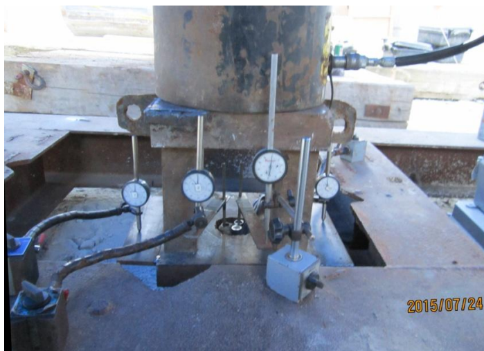
Figure 3. Arrangement of dial gages at the pile head
