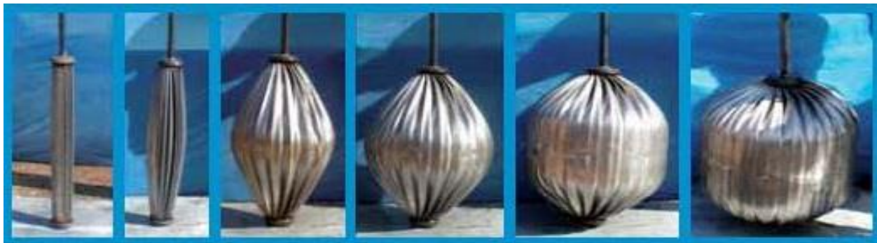
Figure 7: Phases of Expansion of the Expander Body Element
